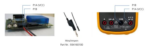
Figure 5: Example – tracking current measurement
