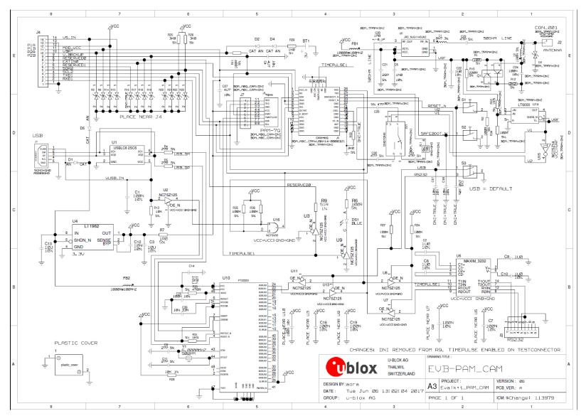
Figure 8: Schematic EVK-7PAM / EVK-M8QCAM / EVK-M8CCAM: DNI=TRUE in the schematic means: Component not installed
