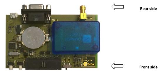
Figure 2: EVK-M8QCAM/M8CCAM evaluation unit - front and rear sides
