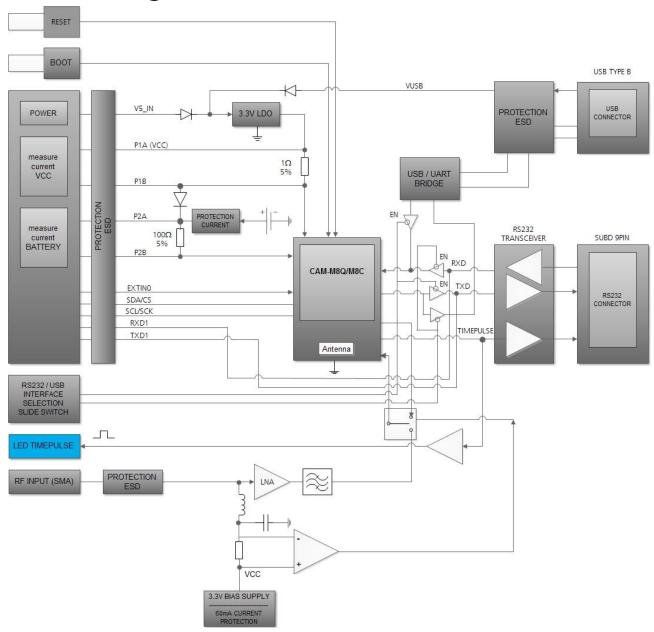
Figure 6: EVK-M8QCAM/M8CCAM block diagram
