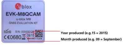
Figure 3: EVK-M8QCAM label with the production date circled in red
