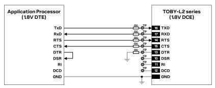
Figure 59: UART interface application circuit with partial V.24 link (5-wire) in the DTE/DCE serial communication (1.8V DTE)
