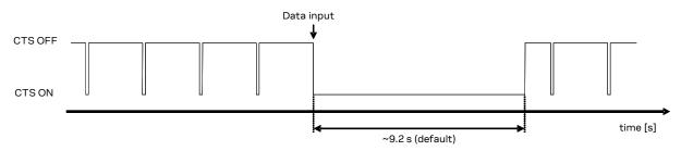
Figure 23: CTS output pin indicates when module's UART is enabled (CTS = ON = low level) or disabled (CTS = OFF = high level)
