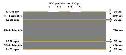
Figure 46: Example of 50  $\Omega$  coplanar waveguide transmission line design for the described 4-layer board layup
