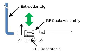
Figure 72: Precautions during RF connector extraction
