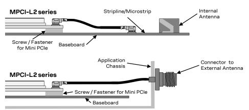
Figure 45: Example of RF connections, U.FL-to-U.FL cable for internal antenna and U.FL-to-SMA for external antenna
