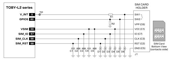
Figure 52: Application circuit for the connection to a single removable SIM card, with SIM detection implemented
