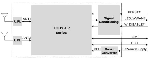
Figure 2: MPCI-L2 series block diagram
