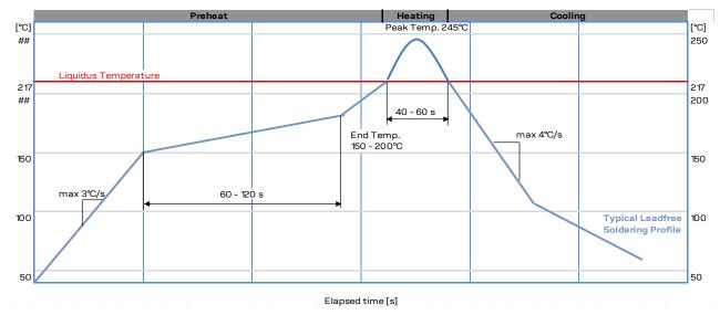
Figure 77: Recommended soldering profile
