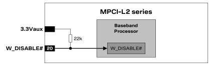
Figure 27: MPCI-L2 series modules W\_DISABLE# input circuit description
