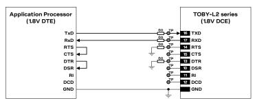
Figure 61: UART interface application circuit with partial V.24 link (3-wire) in the DTE/DCE serial communication (1.8V DTE)
