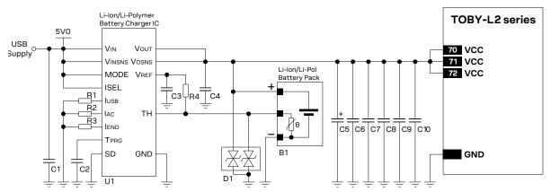
Figure 38: Li-Ion (or Li-Polymer) battery charging application circuit
