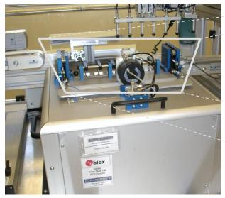
Figure 80: Automatic test equipment for module tests
