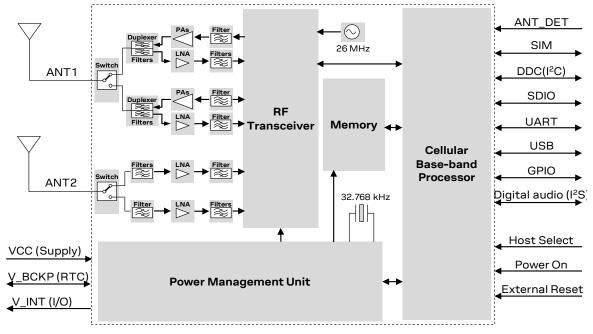
Figure 1 summarizes the internal architecture of TOBY-L2 series modules.
