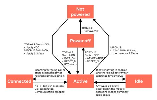
Figure 3: TOBY-L2 and MPCI-L2 series modules operating modes transition
