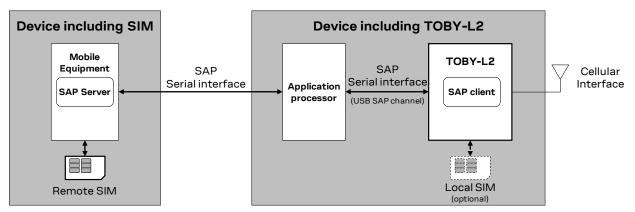
Figure 30: Remote SIM access via completely wired connection
