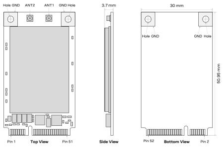
Figure 70: MPCI-L2 series mechanical description (top, side and bottom views)
