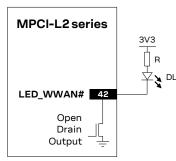
Figure 67: LED\_WWAN# application circuit
