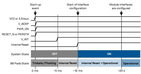
• The module is ready to operate after all interfaces are configured.
