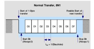
Figure 20: Description of UART default frame format (8N1, i.e. 8 data bits, no parity, 1 stop bit)
