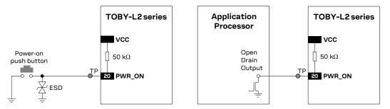
Figure 42: PWR\_ON application circuits using a push button and an open drain output of an application processor
