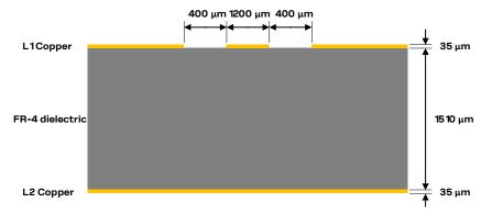
Figure 47: Example of 50  $\Omega$  coplanar waveguide transmission line design for the described 2-layer board layup
