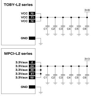
Figure 37: Suggested schematic for the VCC / 3.3Vaux bypass capacitors to reduce ripple / noise on supply voltage profile
