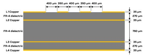
Figure 55: Example of USB line design, with Z $_0$  close to 90  $\Omega$  and Z<sub>CM</sub> close to 30  $\Omega$ , for the described 4-layer board layup
