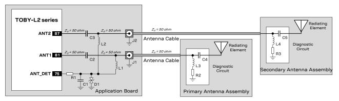
Figure 49: Schematic example for antenna detection circuit on application PCB and diagnostic circuit on antennas assembly
