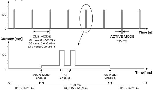
Figure 9: VCC or 3.3Vaux current consumption profile with power saving enabled and module registered with the network: the module is in idle-mode and periodically wakes up to active-mode to monitor the paging channel for paging reception
