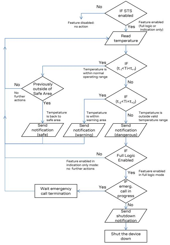
Figure 29: Smart Temperature Supervisor (STS) flow diagram
