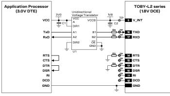
Figure 62: UART interface application circuit with partial V.24 link (3-wire) in DTE/DCE serial communication (3.0 V DTE)
