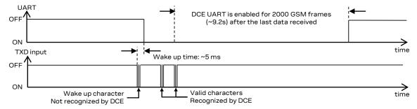
Figure 25: Wake-up via data reception with further communication
