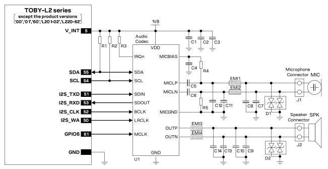
Figure 64: I2S interface application circuit with an external audio codec to provide voice capability
