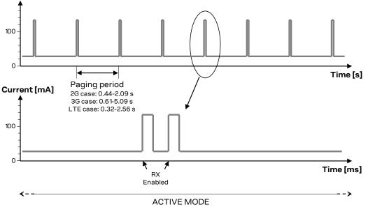
Figure 10: VCC or 3.3Vaux current consumption profile with power saving disabled and module registered with the network: active-mode is always held and the receiver is periodically activated to monitor the paging channel for paging block reception
