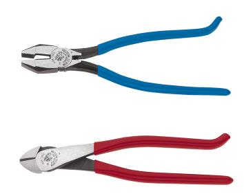
The Ironworker's Kit is a 2-Piece Pliers set that includes a heavy-duty side-cutter and angled-head diagonal cutter, both used to cut soft annealed rebar tie wire. The side-cutters (Cat. No. D2000-7CST) twist tie wire and feature heavy-duty cutting knives for ASCR, screws, nails, and most hardened wire. The diagonal-cutters (Cat. No. D248-9ST) have an angled head to cut tie wire in confined spaces.
