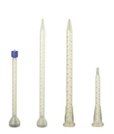
Static mixers connect to the end of dual-part syringes or cartridges and mix two-component materials. Connection to the material is either bell or bayonet style, and the dispensing end may be Luer Slip, Luer Lock, or stepped.
