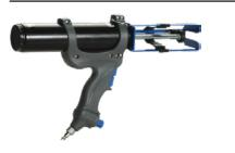
Dual pneumatic gun with a 200 ml capacity for various two part applications. The ratio has several different variations, of 1:1, 2:1, 4:1 and 10:1 with the kits included. It has a twist and lock plunger feature to easily switch between ratios. This unit has an adjustable air regulator at 100 psi and the maximum output of this gun is 145 psi. Nominal thrust 484 lbs.
