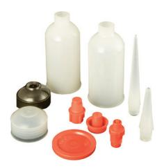
Cartridges are an alternative product when syringes have too small of a capacity. Cartridges are available in low or high density and offered in three different capacities (2.5oz., 6oz. and 12oz.). Cartridge accessories include plunger wipers, end caps and threaded plugs. 1/4" threaded nozzles screw into the cartridge for bead and dot dispensing. Dispensing nozzles are used in conjunction with cartridges when the application requires a reservoir larger than a syringe.
