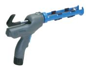
Powered by a 12 volt lithium ion battery pack (battery and charger included) for dispensing standard 10.3 oz & 29 oz. cartridges. It has a one hour charge time for quick charging, and a long lasting battery. The maximum force of this gun is 475 lbs., and has variable speed control.
