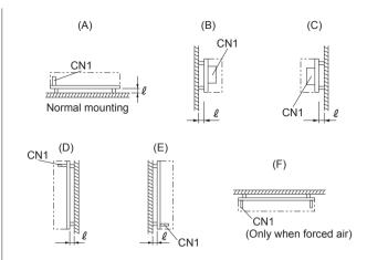
■In case of metal chassis, keep more than 8mm for the part of  $\ell$  to insulate between lead of component and metal chassis. If it is less than 8mm, insert the insulation sheet between power supply and metal chassis.
