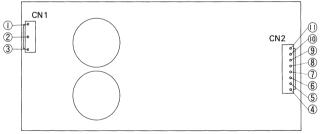
1)Frame ground 2AC(N) 3AC(L) **4**V1 Output ⑤V1 Output 6G1(V1) GND
