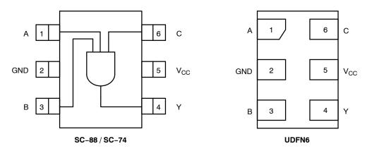
Figure 2. Pinout (Top View)
