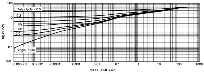
Figure 13. Thermal Characteristics
