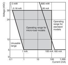
The above diagram is for standard conditions (+5°C to +35°C, 40% to 70%RH). Since the values vary depending on the operating environment conditions, contact your OMRON representative for further details.
